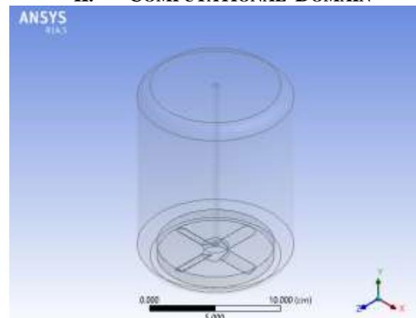
Figure 1: Geometry of Stirred Tank
