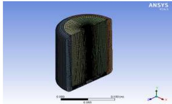
Figure 2(b) Half-sectional view for stirred tank with mesh
