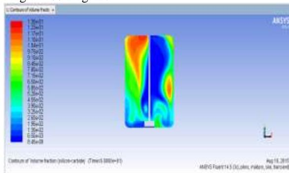
Figure 4 : Contours of volume fraction of Silicon-Carbide for 200 rpm
