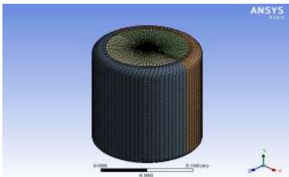
Figure 2(a) : CFD Meshes for stirred tank.
