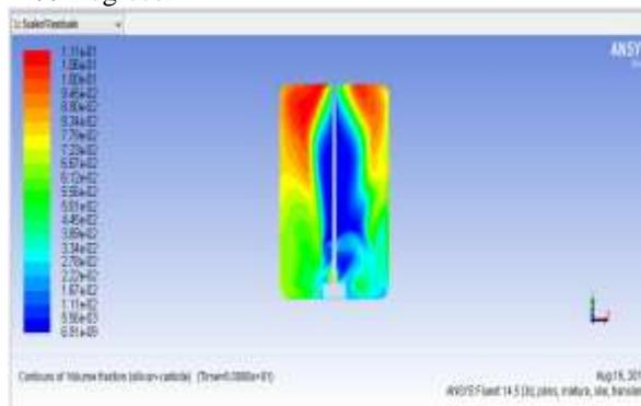
Figure 6 : Contour of volume fraction of Silicon-Carbide for 400 rpm
