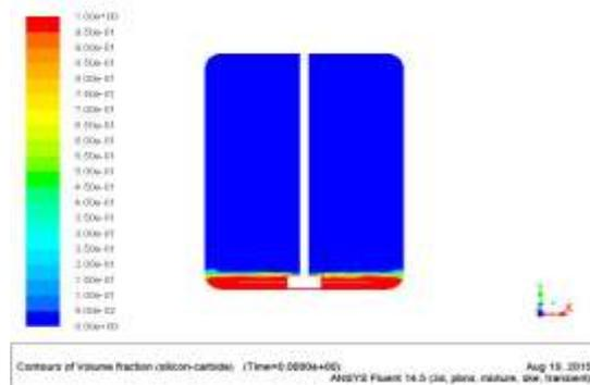
Figure 3: Initial Volume Fraction of Silicon-Carbide at 0<sup>th</sup> seconds
